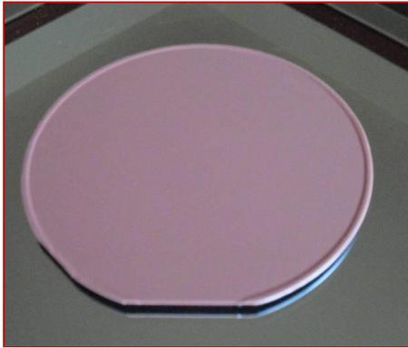
A cleaning wafer to remove dusts or particles on wafer chucks. A polymer pasted on the surface of a silicon wafer absorbs dusts or particles when it contacts with the chuck. Customers can realize the effect of the performance of the CCW by carrying it like as same as production wafers.
