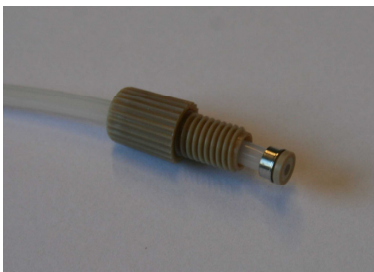
Figure 3.6, Properly assembled microfluidic connection.
