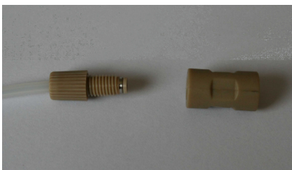
Figure 3.5, Tighten the nut by hand in the union and check the result.
