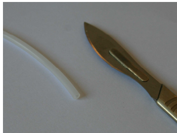
Figure 3.2, ETFE tube end after it is cut.
