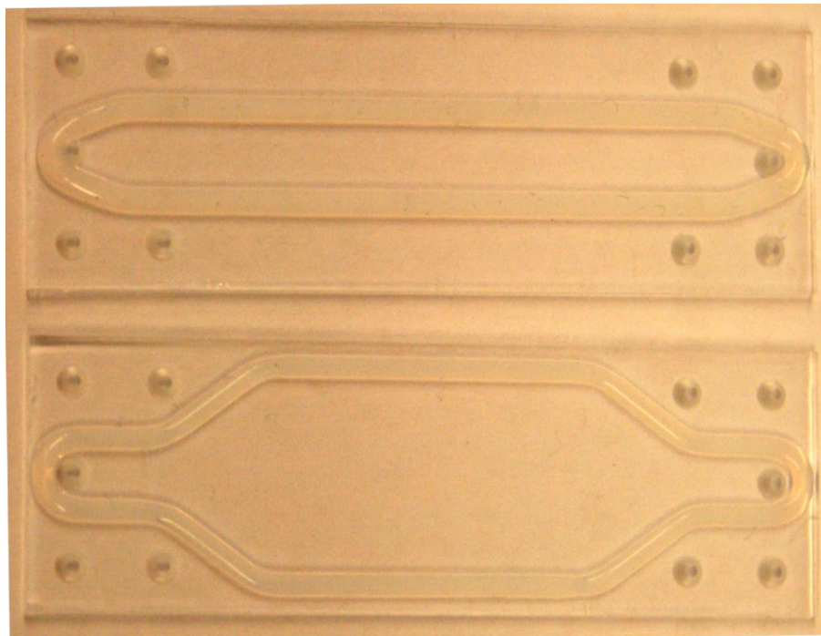
Figure 1: Designs of the two standard layouts, straight flowcell and extended flowcell. The dimensions of the glass slides are 15 mm x 45 mm.
